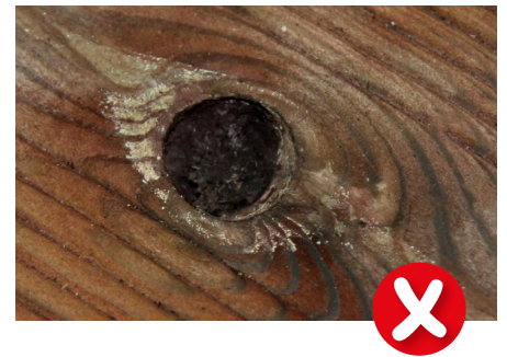
Knot holes – not permitted from 10 mm
