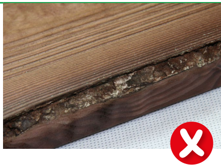
Knot breakouts – up to 20% permitted in intermittent cases
